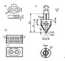
Fig.2 Model diagram (a) form, (b) conical stem, (c) for the knocking-out test by PN-85/11005(10)
