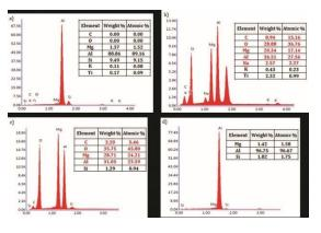
Fig. 7 SEM-EDS results of the sample taken from the surface of diamond cut wheel (sample no:2): (a) selected area 1, (b) selected area 2, (c) selected area 3, (d) EDS spot 1
