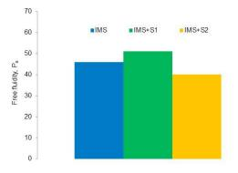
Fig.5 Free fluidity of moulding sands with the Geopol® geopolymer binder and relaxation additives S1 and S2
