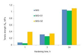
Fig.4 Dependence of the tensile strength of the Geopol® geopolymer binder, after curing, for sands with relaxation additives S1 and S2
