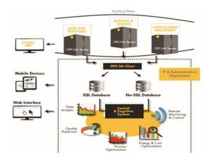
Fig.2 Connectivity and smart monitoring of the foundry process to elaborate OEE and apply quality predictive models
