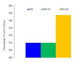
Fig.6 Permeability of moulding sands with the Geopol® geopolymer binder and relaxation additives S1 and S2
