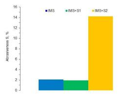
Fig.7 Abrasiveness of moulding sands with the Geopol® geopolymer binder and relaxation additives S1 and S2
