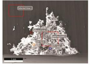
Fig.8 EDS analysis regions on the surface of diamond cut wheel (sample no:3)
