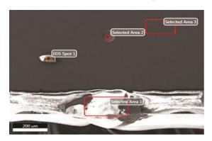
Fig.4 EDS analysis regions on the surface of diamond cut wheel (sample no:1)
