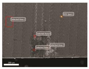
Fig.6 EDS analysis regions on the surface of diamond cut wheel (sample no:2)
