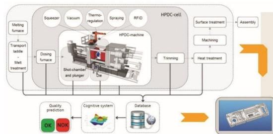
Fig.1 Multi-stage and devices of HPDC cell connectivity of ICT platform for smart monitoring of the process and quality predictive models
