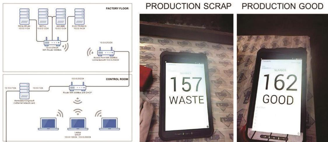
Fig.4 LAN network connection and real time prediction of waste and good castings
