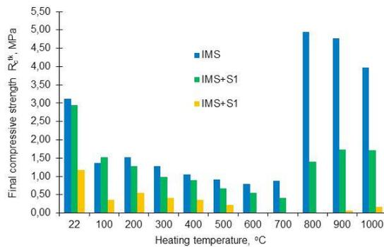
Fig.1 Final compressive strength of moulding sands with inorganic binder (IMS – without additive, IMS+S1, IMS+S2 – with relaxation additive)
