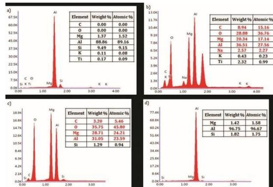
Fig.7 SEM-EDS results of the sample taken from the surface of diamond cut wheel (sample no:2): (a) selected area 1, (b) selected area 2, (c) selected area 3, (d) EDS spot 1
