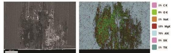
Fig.10 Elemental mapping results of 'sample 2' taken from the region of inclusions
