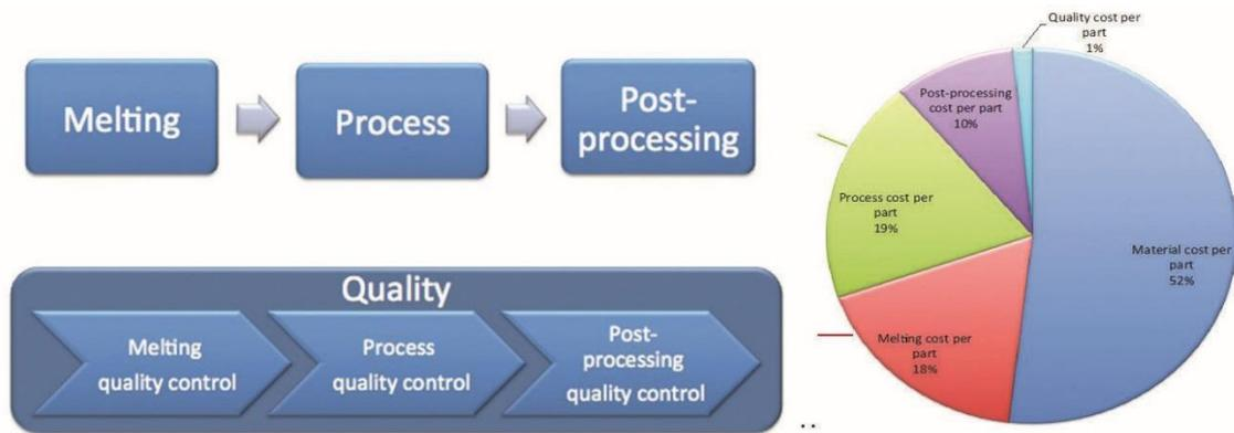
Fig.5 Cost centre approach for the diecasting process and example of cost model application
