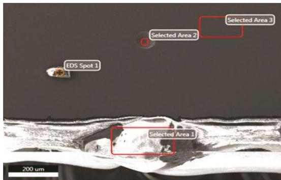
Fig.4 EDS analysis regions on the surface of diamond cut wheel (sample no:1)
