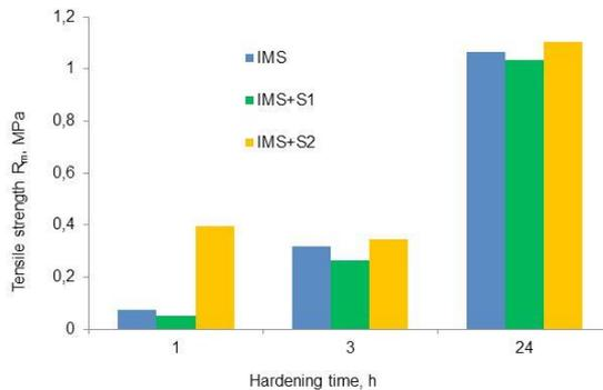
Fig.4 Dependence of the tensile strength of the Geopol® geopolymer binder, after curing, for sands with relaxation additives S1 and S2
