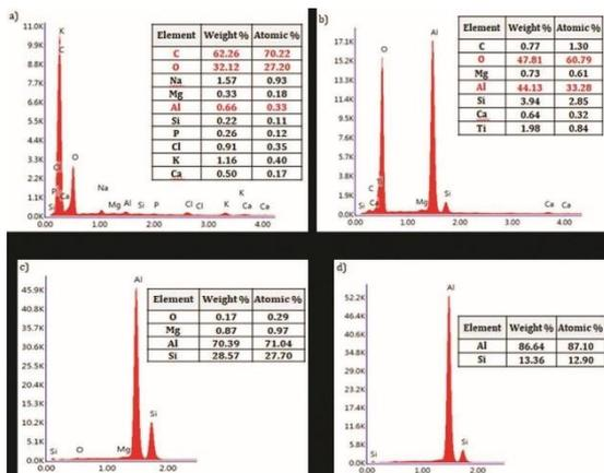
Fig.5 SEM-EDS results of the sample taken from the surface of diamond cut wheel (sample no:1): (a) EDS spot 1, (b) selected area 1, (c) selected area 2, (d) selected area 3
