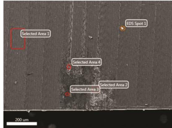
Fig.6 EDS analysis regions on the surface of diamond cut wheel (sample no:2)
