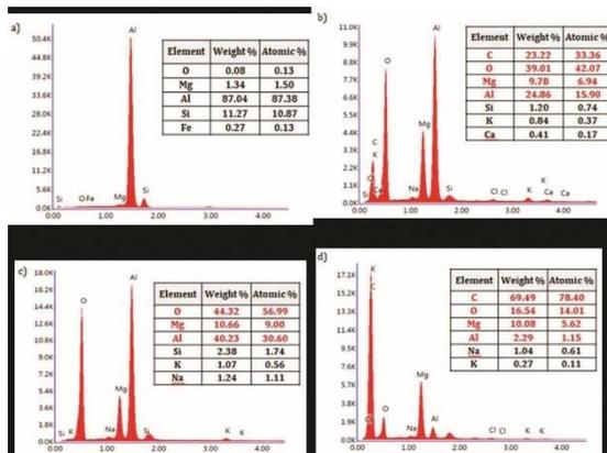
Fig.9 SEM-EDS results of the sample taken from the surface of diamond cut wheel (sample no:3): (a) selected area 1, (b) selected area 2, (c) EDS spot 1, (d) EDS spot 2
