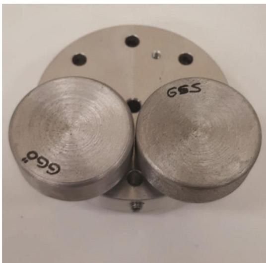
Fig.3 Cast samples obtained from different steps of the production process of aluminium alloy
