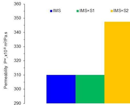
Fig.6 Permeability of moulding sands with the Geopol® geopolymer binder and relaxation additives S1 and S2
